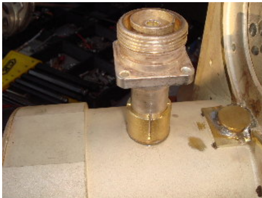
Cavity with the old outcoupling closed and the new one created
